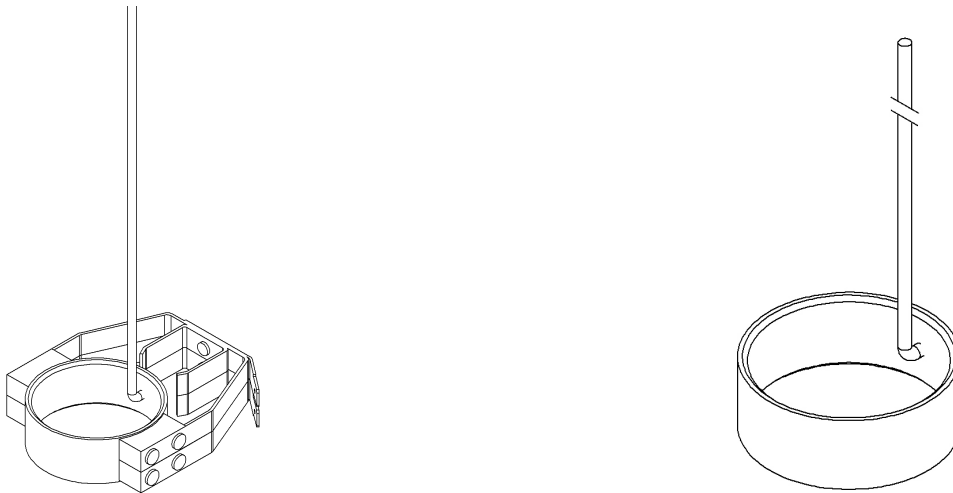
Figure 14: Type 45/2 current collector with slip ring and stranded wire
