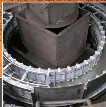
Energy Guiding Chains on circular stacker/reclaimer - complete rotational movement
