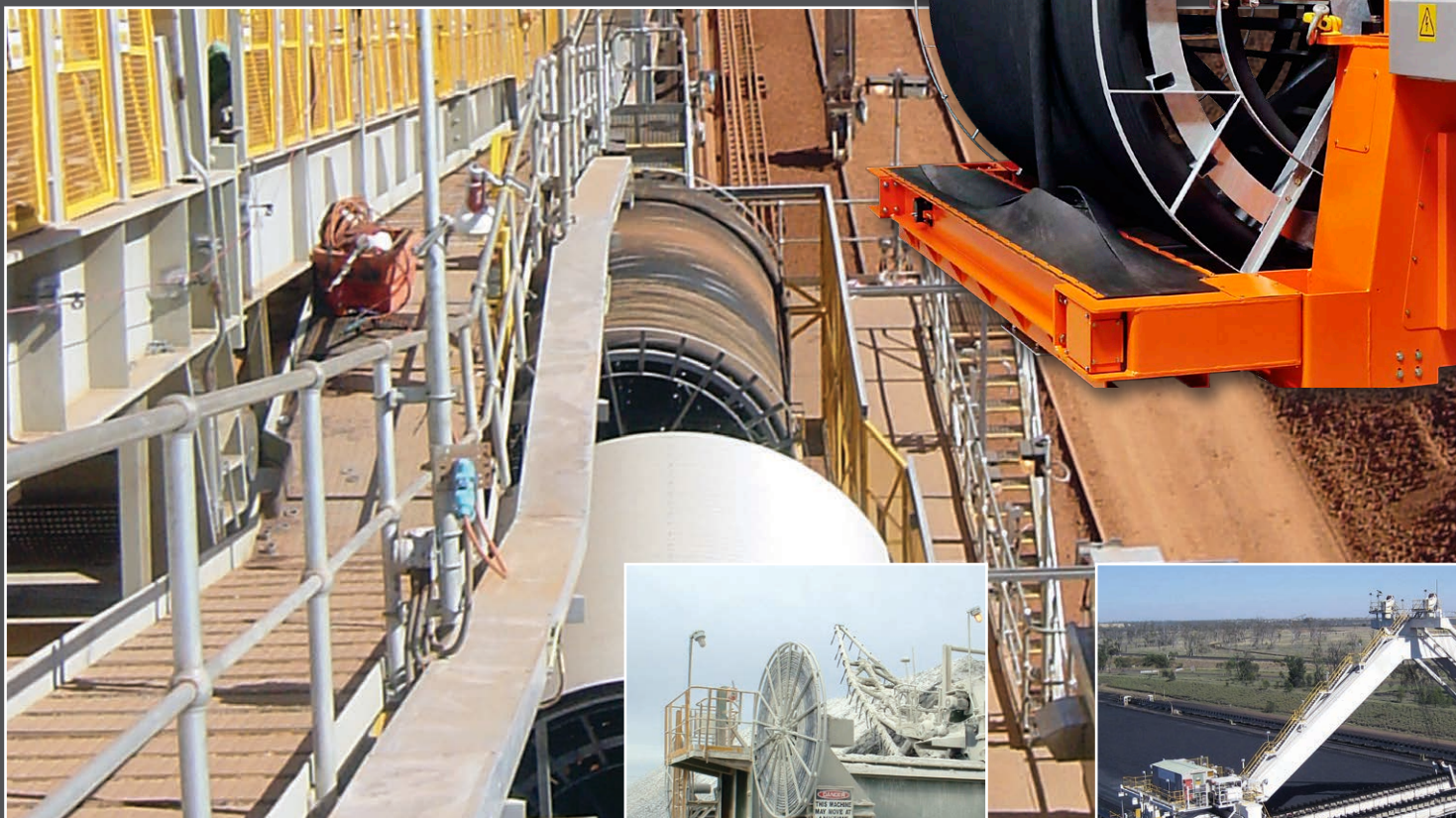
Level Winding Reel on a Stack Rake, USA Travel Length: 1500 m
