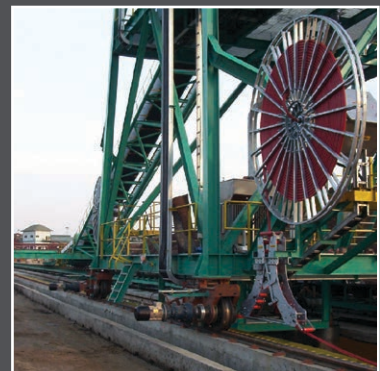
Motor Driven Cable Reel on a Stacker/Reclaimer, Thailand, Travel Length: 380 m
