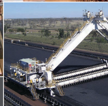
Level Winding Reel on a Portal Reclaimer, Australia Travel Length: 680 m
